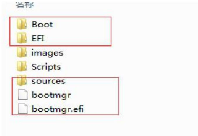
4. The second USB disk makes the System Disk. When formatting the USB disk, the file system is selected as [NTFS] format, and the label is changed to WINPE, then click [Start].
